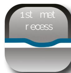
X-line also has a 1st metatarsal recess freeing the 1st metatarsophalangeal joint from early and high pressure in stance to allow good sagittal motion as the foot accelerates towards the next step.
